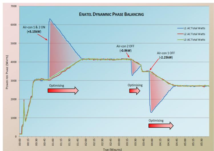
This form of phase balancing has been patented by Enatel.
