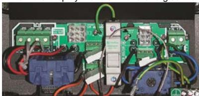
**Note, the above is only on older versions.** Earlier versions of the 1.5-3.8kW models incorporate a separate earth fuse
