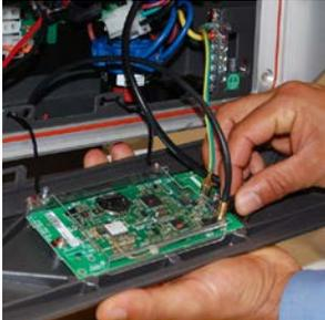
**Disconnecting Display Module Connectors**
