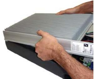
**Removing the Inverter Module**
