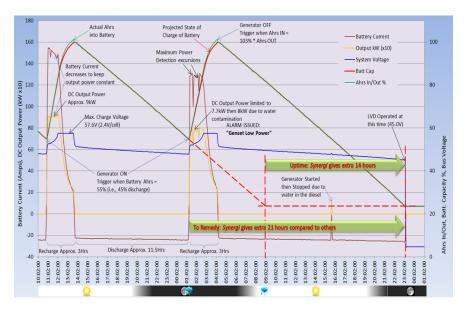
• At the time of the second start, it can be seen from the plot that the DC output power had to be limited to under 8kW. At this time, a Low Genset Power alarm could be raised to alert the NOC that there was a problem at site. Due to the D<sup>2</sup>GO (dynamic diesel generator optimisation) functionality, SYNERGi kept the genset operating when it would normally have stalled, thus being able to fully recharge the battery.
