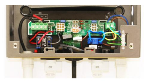
Wall Mount Sample Wiring - 1.5 to 3.8kW Models.
