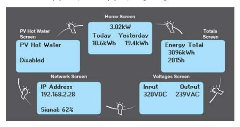
**Display Module Navigation** (note: screen text above is indicative only. Actual screen text will vary depending on model and system configuration)
