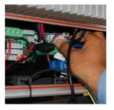
Disconnecting Inverter Module Plugs
