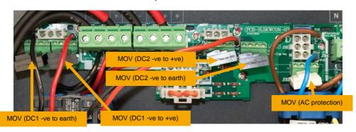
Installer Serviceable Components 4.0/5.0kW Inverter Models
