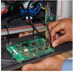
Disconnecting Display Module Connectors
