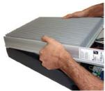
Removing the Inverter Module
