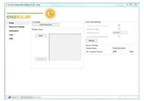
If a Wi-Fi inverter version is being installed. click the Scan button on the Setup page. A list of wireless networks within range of the inverter will be displayed. Select the customer's wireless network from the list and click the Connect button. The Inverter Configuration Software will prompt for any required Wi-Fi passwords.
