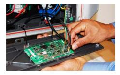
Display Module (Wi-Fi) with Connections
